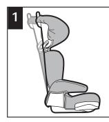
Backrest has 2 positions, upright and semi-reclined. The semi-recline position is to be used only to install the child restraint flush against the back of the vehicle seat back, if needed.
